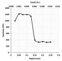
Capable of case depths up to 0.008" (0.2 mm). Stainless alloys are rich in nitride forming elements (most notably Cr), which results in high hardness, but limited case depth.
