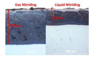
Gas nitriding is not only capable replicating the results of conventional salt-bath (liquid) methods, but can also be tailored to achieve deeper case depths.
