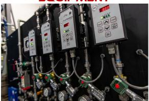
You are only as good as your equipment! Our state-of-the-art nitriding furnaces utilize temperature and atmosphere sensors to control processing conditions in real time. Closed-loop feedback ensures operating conditions are representative of the recipes prescribed by our expert metallurgists.
