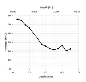
Case depths controlled to ensure they are less than **0.006**" to conform to even the most stringent specifications. Process parameters are computer-controlled to ensure base material hardness is kept below **22HRC**.
