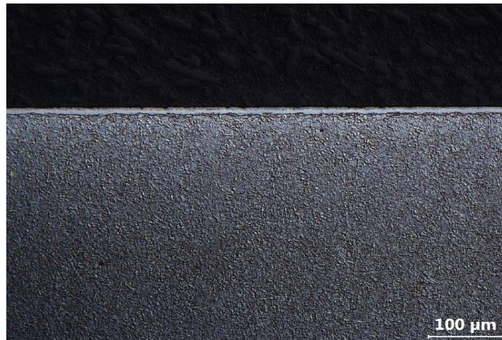
Figure 1: Representative photomicrograph of the hardened section microstructure. DIC Illumination, 3% Nital Etch
